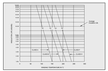
Figure 7-6: Insulation Life vs. Temperature
