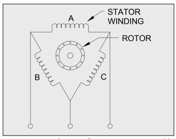
Figure 4-1: Development of a Rotating Magnetic Field
