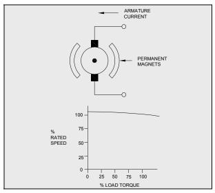
Figure 5-5: Permanent Magnet DC Motor
