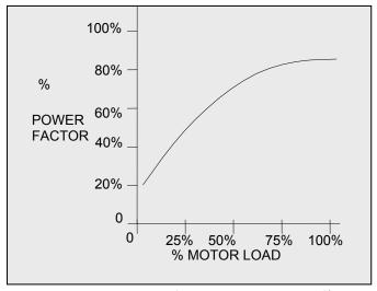
Figure 7-11: Typical Power Factor vs. Load<sup>2</sup>
