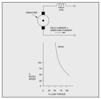
Figure 5-3: Series Field Motor
