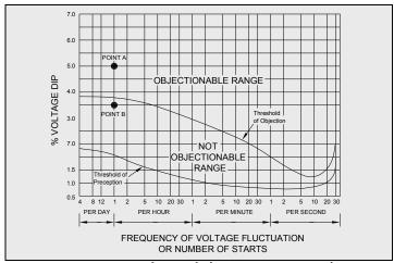
Figure 7-4: Voltage Flicker Curve - Example
