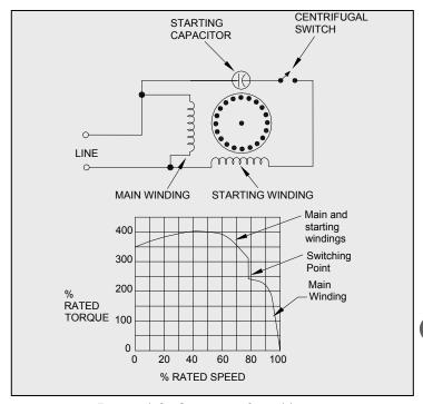
Figure 4-9: Capacitor Start Motor
