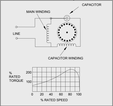
Figure 4-8: Capacitor Run Motor
