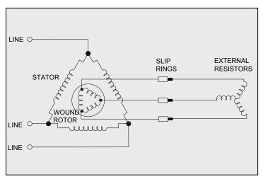
Figure 4-5: Wound Rotor Induction Motor
