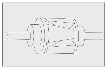
Figure 4-13: Non Excited Synchronous Motor Rotor
