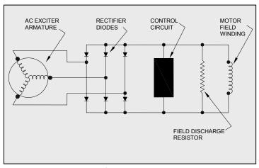
Figure 4-12: Exciter for Brushless Synchronous Motor
