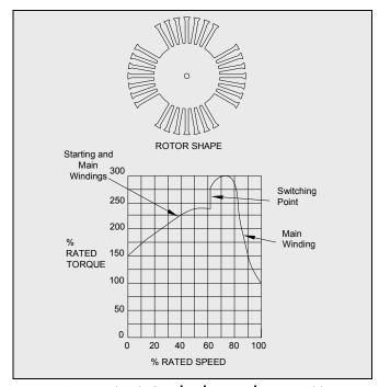
Figure 4-14: Single Phase Reluctance Motor
