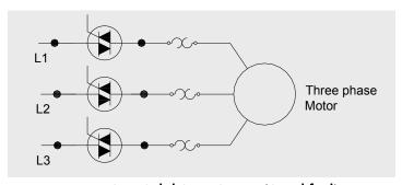
Figure 8-5: Solid State Starter (Simplified)
