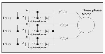
Figure 8-4: Autotransformer Starter
