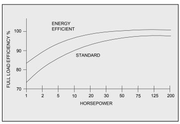
Figure 7-10: Typical Efficiencies of Standard and Energy
