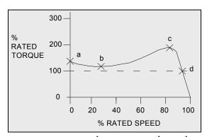
Figure 3-3: Typical Torque-Speed Graph
