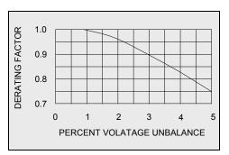
Figure 7-1: 3-phase Squirrel Cage Induction Motors
