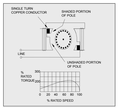
Figure 4-11: Shaded Pole Motor
