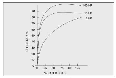
Figure 7-9: Typical Motor Efficiency vs. Load
