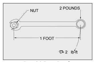
Figure 3-2: Torque Example
