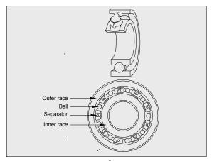
Figure 9-1: Antifriction Bearing
