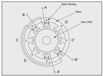
Figure 6-4: Hybrid Motor
