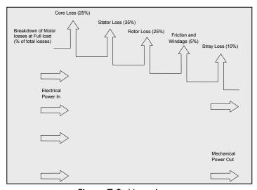
Figure 7-8: Motor Losses
