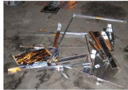
Top row: total unit - 108.9 kg., ferrous metal shell – 42 kg., non ferrous trim – 3.6 kg
