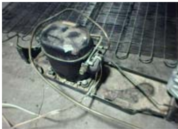
Middle row: ferrous compressor 12 kg, copper and aluminum coils and cooler – 8.6 kg., PVC coated copper wiring - .9 kg., ferrous screws, bolts, fasteners – 2.5 kg.
