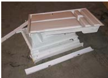
Bottom row: plastic door moldings – 5.4 kg., Other plastic seals and moldings - .45 kg., fiberglass insulation 1.3 kg. Not shown: ferrous door panels, drawers/shelves.
