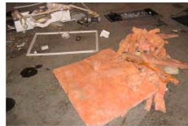
Bottom row: plastic door moldings – 5.4 kg., Other plastic seals and moldings - .45 kg., fiberglass insulation 1.3 kg. Not shown: ferrous door panels, drawers/shelves.
