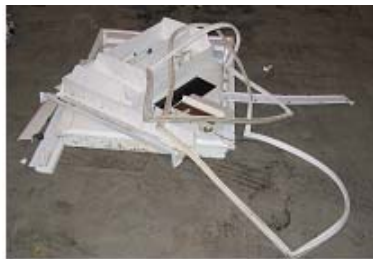
Bottom row: plastic door moldings – 5.4 kg., Other plastic seals and moldings - .45 kg., fiberglass insulation 1.3 kg. Not shown: ferrous door panels, drawers/shelves.
