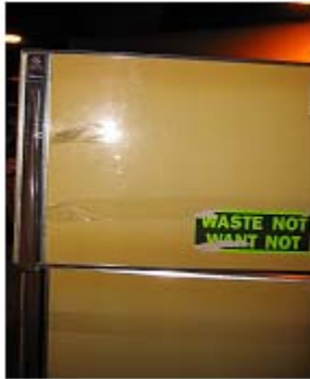
Top row: total unit - 108.9 kg., ferrous metal shell – 42 kg., non ferrous trim – 3.6 kg
