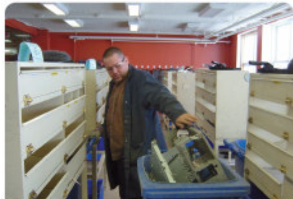
Disassembly tables laid out so that a worker can pick up the components from the back and sort them
