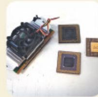
microprocessors (plastic, gold, and ceramic)
