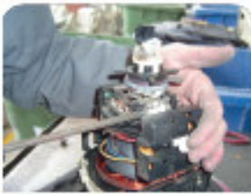
Removing the yoke
