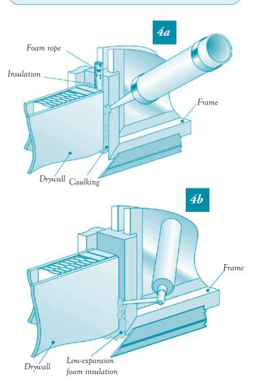
Figures 4a and 4b How to seal behind the window trim Figure 5 Where to weatherstrip a single-hung window
