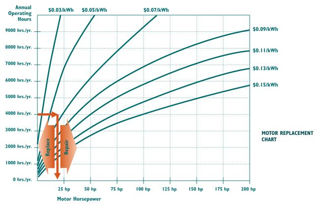
Select the hours that the motor operates and draw a horizontal line until it intersects with the average electric cost curve. Then draw a line down until it intersects the motor size on the x-axis. Any motor size to the left should be replaced with a HEM; any motor size to the right should be rewound.
