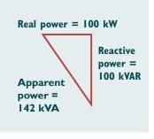
Induction motors are the principle cause of poor power factor. Electric utilities often levy a penalty for power factors that fall below a certain level, typically 90%. Some strategies for correcting poor power factor include
