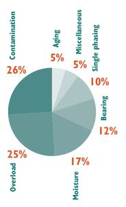
**CAUSES OF MOTOR FAILURE**
