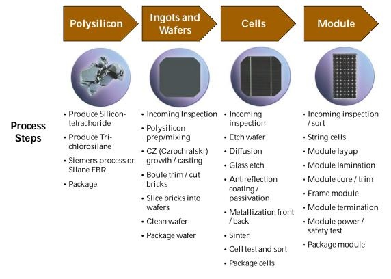
Figure 10 – Process Steps for Crystalline Silicon Module
