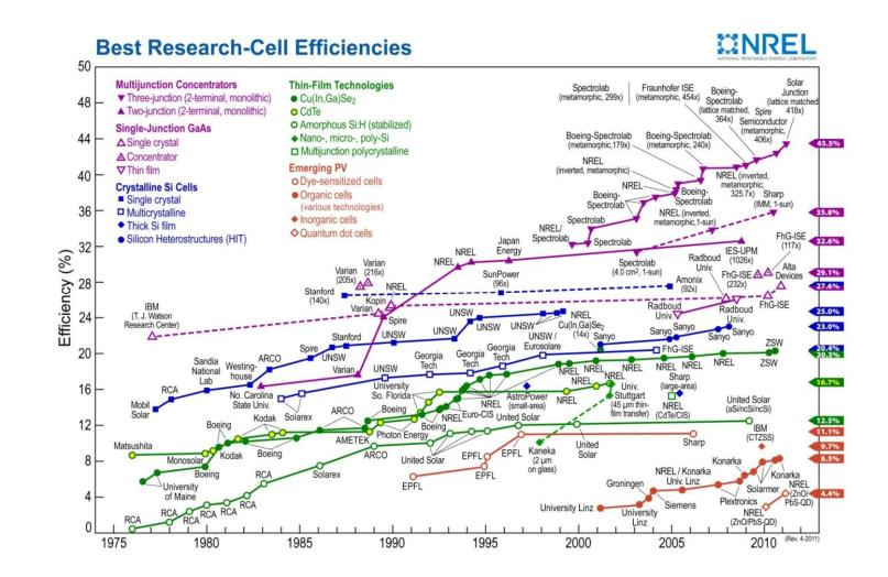
Figure 16 – Global PV Module Technology Overview and Efficiencies Reached
