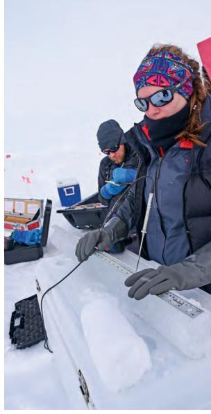
Measuring the temperature of a core of first-year sea ice
