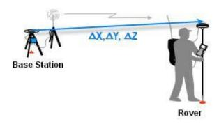
Figure 2-1 Typical RTK Setup.
