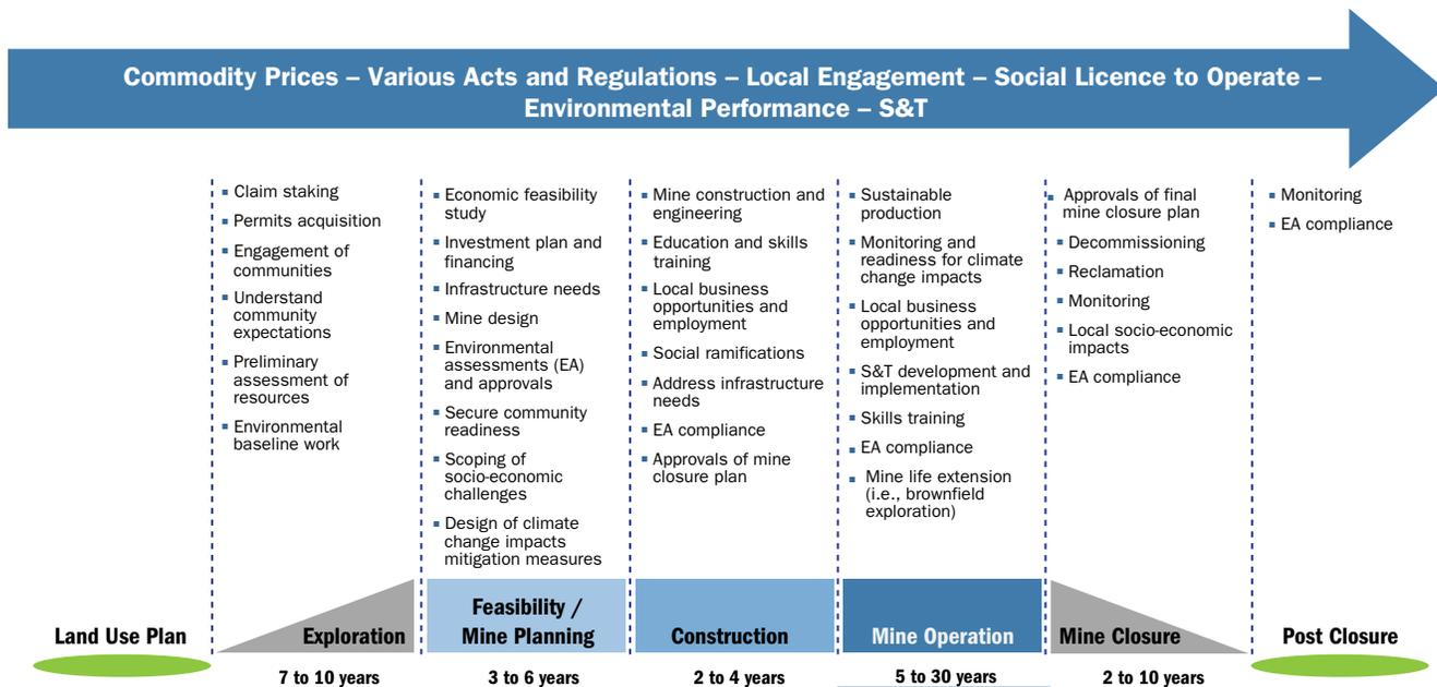
The minerals and metals resource cycle encompasses a process that starts with land-use planning and exploration and follows with mine development, operation, closure, and post-closure monitoring.
