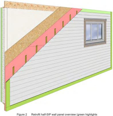
ure 2 Retrofit half-SIP wall panel overview (green highlights indicate site-applied perimeter joint/tie-in components)
