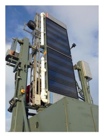
Figure 1: BIPVT collector prototype designed by KNU on CanmetENERGY's PVT Testing Facility
