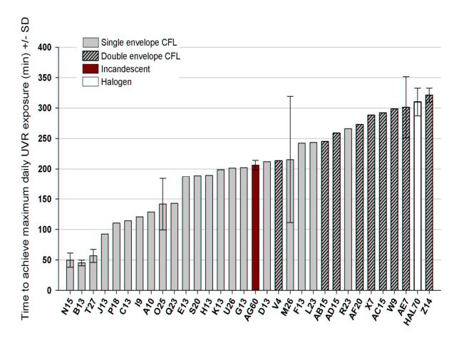
Figure 1. Calculated UVR T<sub>max</sub> for various bulbs at an exposure distance of 3 cm.
