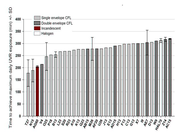
Figure 2. Calculated UVR  $T_{max}$  for various bulbs at an exposure distance of 30 cm.
