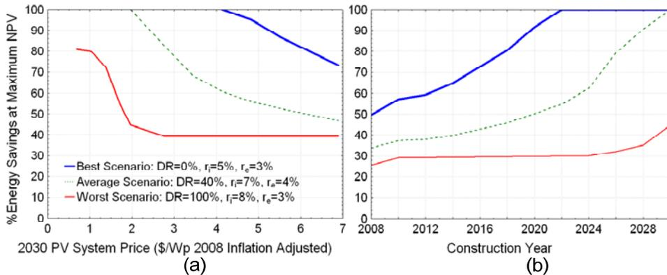
Figure 4 Optimal energy saving solution to maximize the NPV as a function of (a) the 2030 PV system price (b) the house construction year
