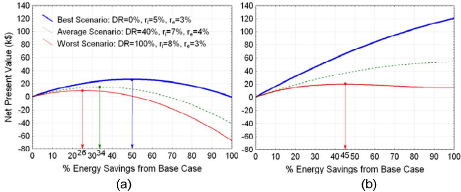
Figure 2 Net present value for houses with variable levels of energy savings built in (a) 2008 (b) 2030
