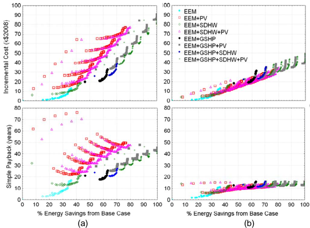
*Figure 1 Incremental cost and simple payback of using (a) actual costs (2008) (b) future cost (2030)*
