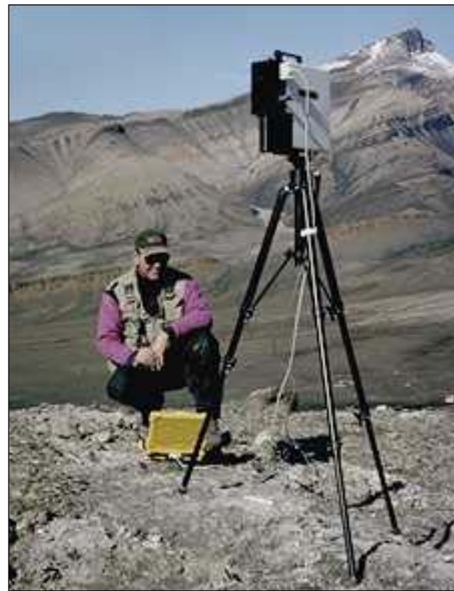
Figure 2. Field spectrometer in operation over a bedrock target in the High Arctic (Photo: Paul Budkewitsch)
