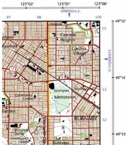
As an example, the position of the sportsplex located in the top right corner of 92-G/3 Lulu Island of British Columbia is located in UTM Zone 10 and the coordinates are 498400m.E. and 5453100m.N. The same position can also be described using geographic coordinates 123°01'W longitude, 49°14'N latitude.
