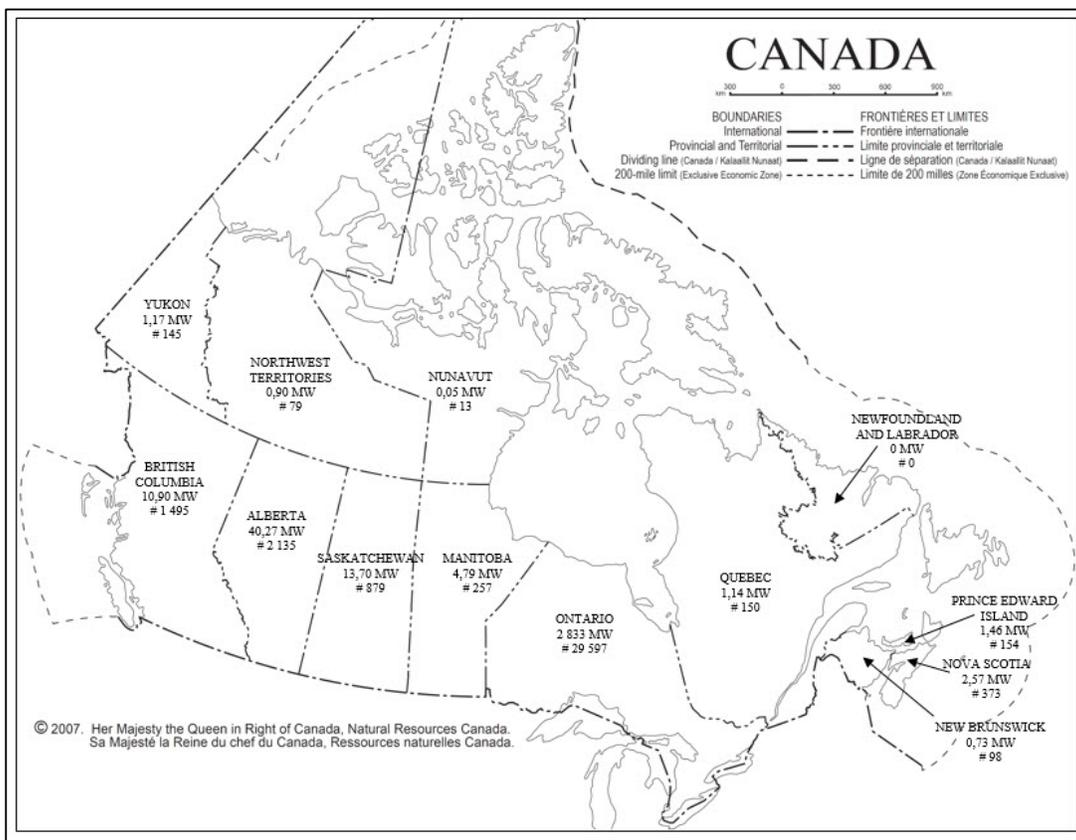
**Figure 1:** Map showing the Canadian provinces and territories, grid-connected PV power capacity (reported in DC megawatt peak, MW<sub>p</sub>), and the number of utility interconnected PV systems as of December 31, 2017.
