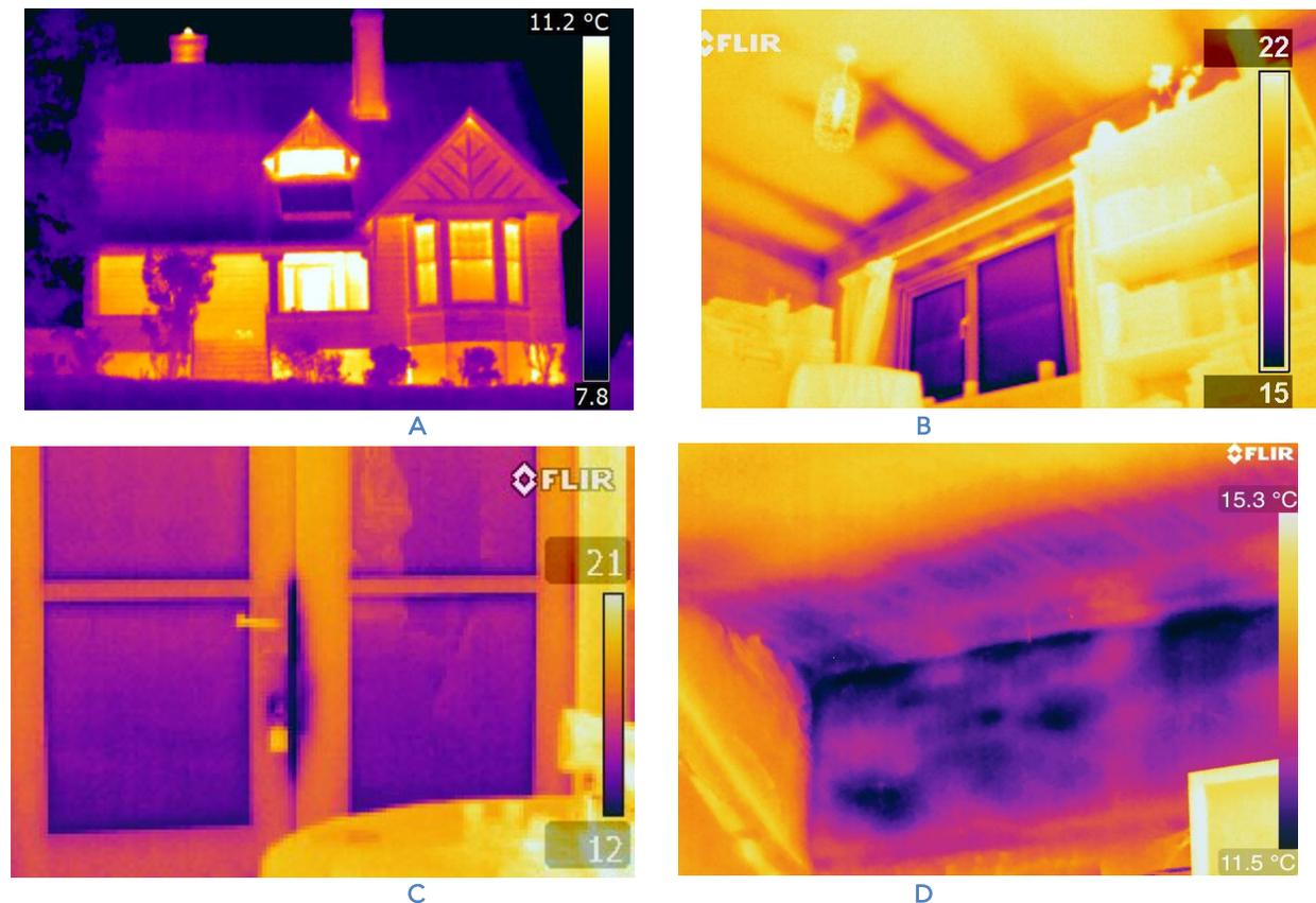
Figure 1: a) Thermal image of exterior front of a house in Vancouver (City of Vancouver); b) An example of conduction heat loss and thermal bridging; c) An example of ventilation heat loss from the interior of the home; d) An example of moisture ingress.
