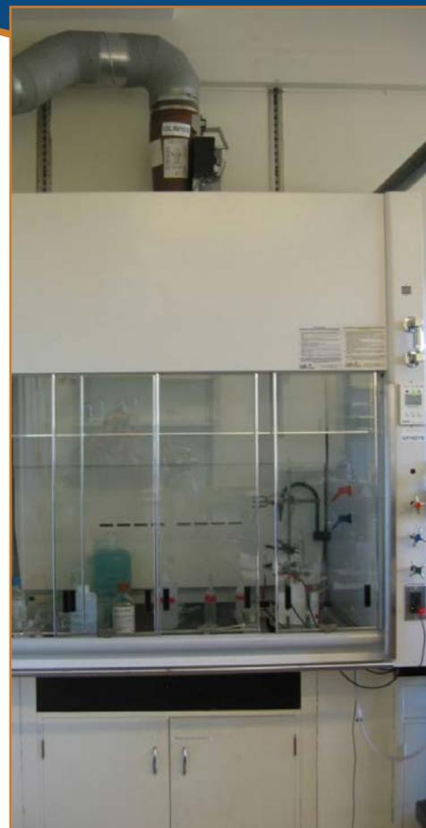
**New high efficiency/low airflow fume hood**
