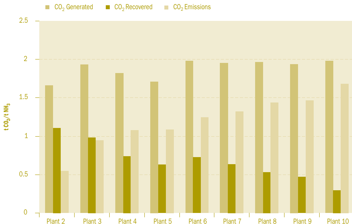
Figure 4: CO 2 Recovery and Emissions – Specific Basis
