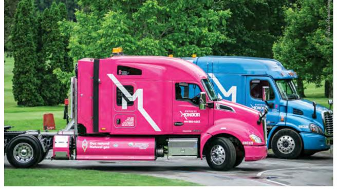
Kenworth T680, Cummins engine ISX12N, Eaton autoshift transmission, Agility tank with 210 DGE capacity, painted for the Quebec Breast Cancer Foundation
