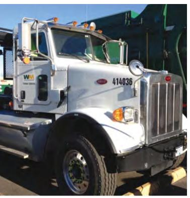
Waste Management roll-off truck with a CWI 12-litre engine
